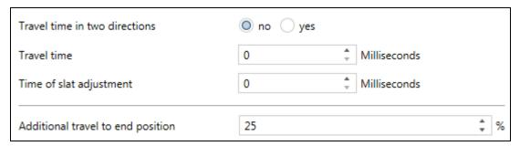
**Travel time in two directions** – defines how the blind travel time will be determined:
