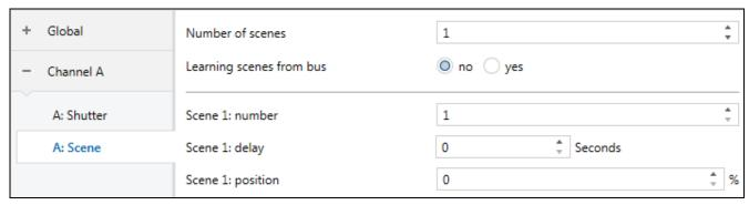
**Number of scenes** – number of scenes assigned to the channel (up to 8). For each activated scene, parameters are displayed which allow you to define for slat-type blind reaction to the scene.
