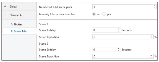
**Number of 1-bit scene pairs** – the number of 1-bit scene pairs assigned to the channel (up to 4). For each activated pair, the "Call scene 1-bit (X/Y)" communication object (where: X/Y = 1/2, 3/4, 5/6, 7/8) is enabled and parameters are displayed which allow you to define blind/shutter reaction to the scene.
