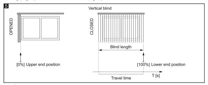
The "Vertical blind" is only supported by the KNX-BSA12L module.
