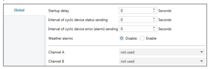
**Startup delay** – time period by which the module startup will be delayed after power-on (0 – 65535 [seconds]). Value "0" will disable the delay.
