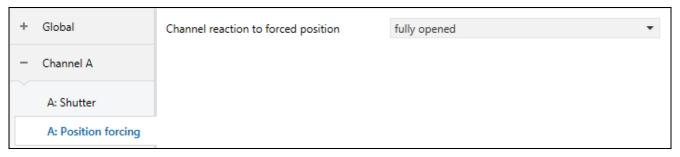
**Channel reaction to forced position** – position to which the blind/shutter will be set in response to a change of state of the "Forced position" communication object (fully opened / fully closed / stop).
