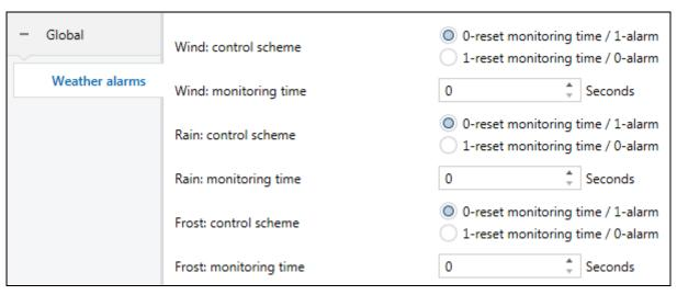
Wind: control scheme – value of the "Wind alarm" object activating telegram:
